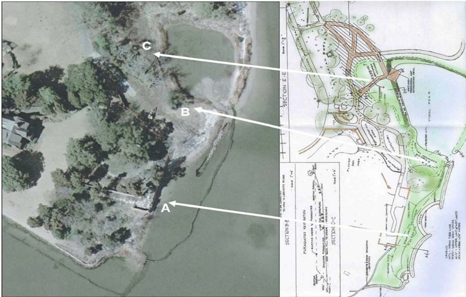
Figure 3: Diagram showing the approximate locations of the different phases of Restoration as part of the Hermitage Living Shorelines Restoration Project. 300 linear feet of shoreline were protected through the creation of a living shoreline at Site A. Removal of an invasive strand of Phragmites and replacement with 5000 SF of tidal marsh took place at Site B. Removal of approximately 400 cubic yard of debris and planting of native plants restored 7500 SF of tidal wetlands at Site C.
